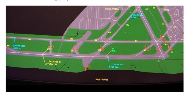
**Graphic No. 1**: Captured A-SMGCS image showing EI-EFF (Callsign 342) and EI-DHA (Callsign 45TR) at their closest point (807 m). (AAIU Note: a number of taxiway identifier labels have been re-positioned for clarity)
